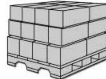
Avoid misalignment, which can reduce compression strength by up to 30%.
